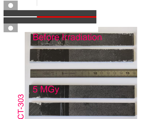
Glue DCB for Mode I fracture Tests
