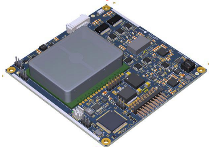
Voltage Distribution Board
