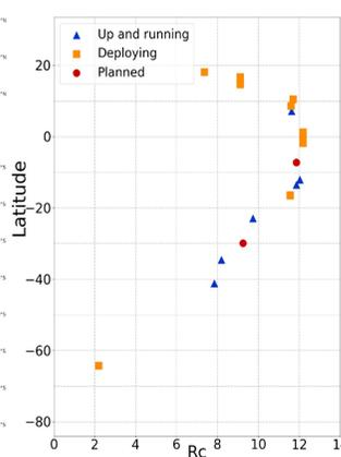
The Latin American Giant Observatory (LAGO) constitute a **Water Cherenkov Detector (WCD) network** through Latin America, with large variation of altitudes and rigidity cut offs and **different detector geometries**.
