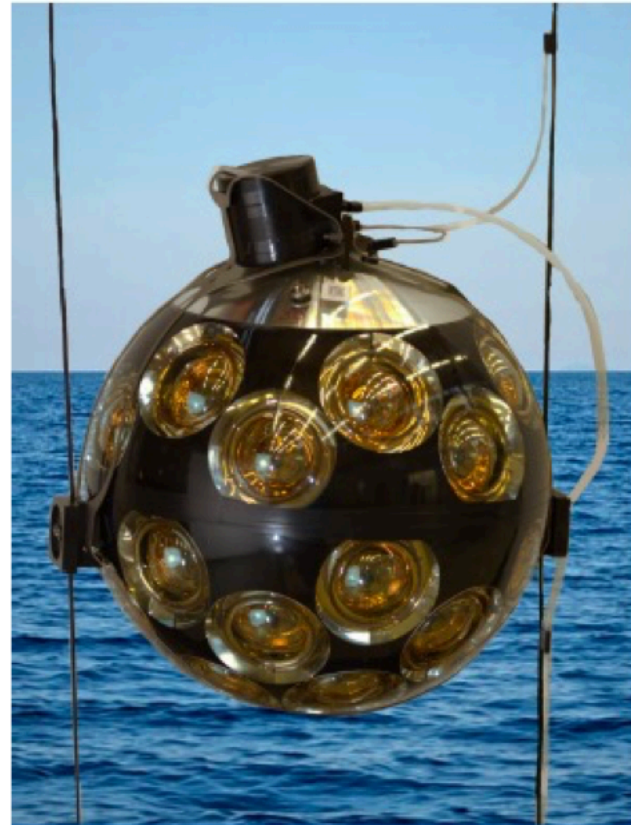
1 optical module = 31 photomultiplier tubes
