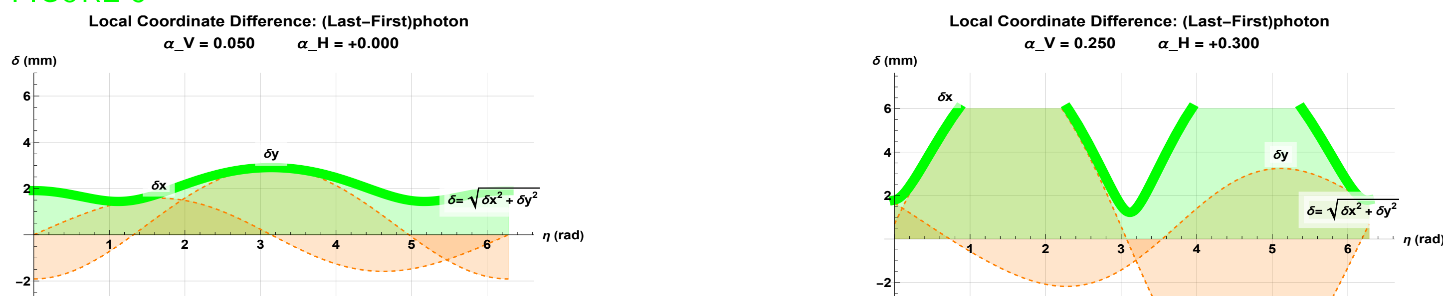
Photon hits for particle trajectory at small (left) and large (right) angles with respect to the beam-line.
