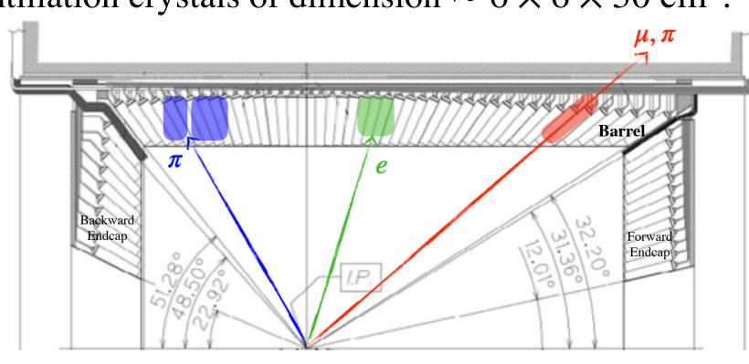
The dominant interaction in the ECL for  $\mu$ and  $\pi$  in  $p_T \in [0.28, 0.9]$  GeV/c is ionization. Additionally  $\pi$  can strongly interact with nuclei. Electrons generate EM showers depositing the majority of their energy in the ECL.
