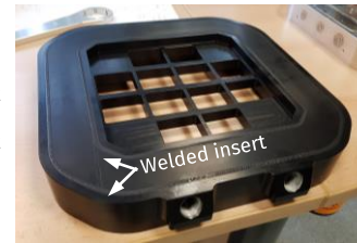
Focal plane plate test piece with welded insert
