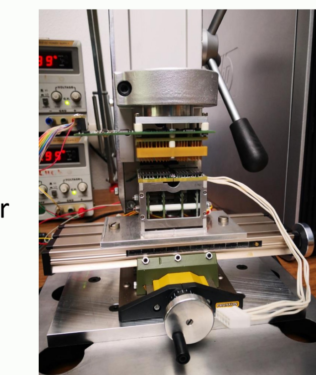
Figure 9: Test station used for the BBs QA.
