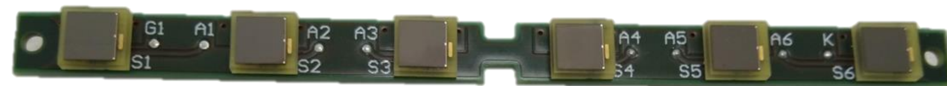
Prototype 6-channel array based on NUV-HD-Cryo fabricated at Lfoundry and packaging developed by FBK.
