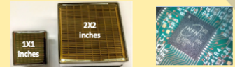
Figure 3: Left: Hamamatsu MaPMTs the R13742 (R-Type) on the left and R13743 (H-Type) on the right. Right: CLARO ASICs.
