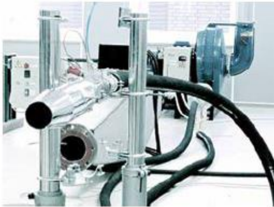
Test rig to determine acoustic parameters of micro-structured materials at high flow speed and high temperature (a) and Schematic of acoustical to mechanical power conversion and final energy harvesting (b)
