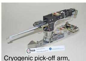
Cryogenic pick-off arm, positioning accuracy 120µm
