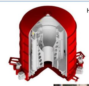
HARMONI Cryostat cut-through (4m high, 3.5m diameter)
