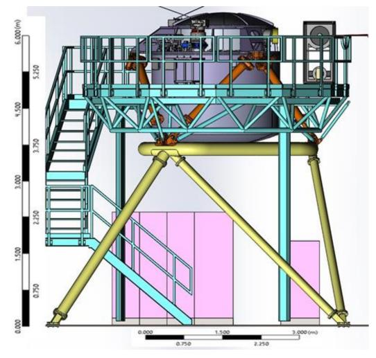
Warm Support Structure (WSS) is the cryostat and Nasmyth platform interface with 3 sub-structures:
