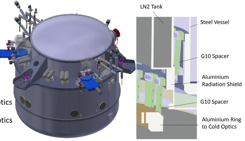
Cryostat Wall Design
