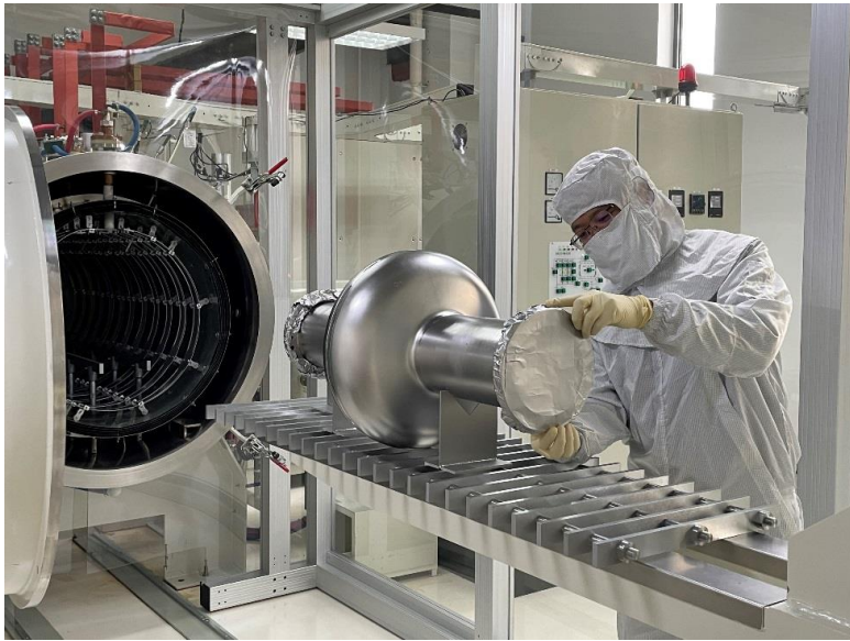
Mid-T furnace baking of 650 MHz single-cell cavity
