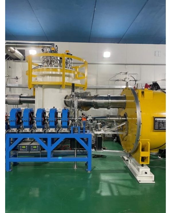
Downstream beamline and valve box connection
