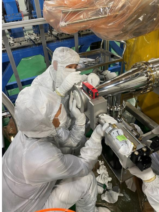
Downstream HOM absorber, taper, ion pump, gate valve
