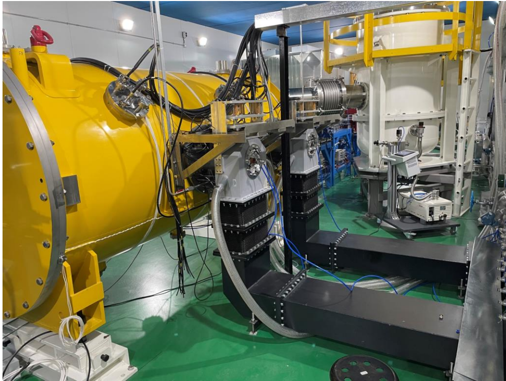
Input coupler warm part, doorknob, waveguide
