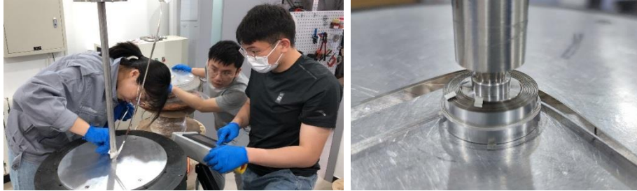
Coil winding of the IBS double pancake solenoids with 20-mm inner diameter
