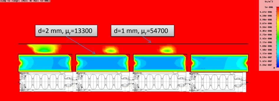
**B-Field** Туре Component Abs Plane at x 0 0.00389417 Us/m<sup>2</sup> at -2.92938e-014 / 480.947 / 3039.33 Maximum-2D
