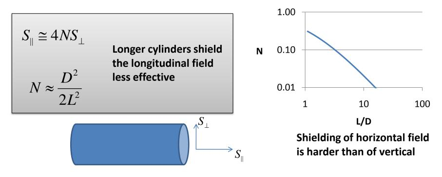
S: Shielding factors μ: Permeability of material d: Thickness of sheet D: Diameter of cylinder L: Length of cylinder N: Demagnetization coefficient
