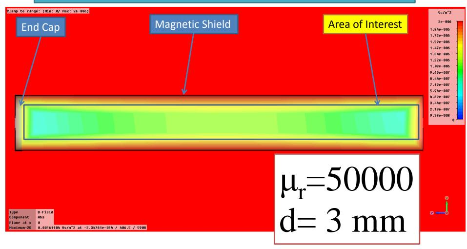
If the whole cryomodule shares one shield a maximum field value of approximately 1  $\mu T$  can be achieved for  $\mu_r\!=\!50000$  and d=3 mm
