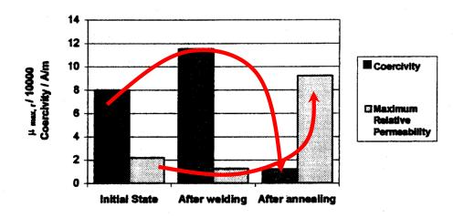
Note: The properties of the initial state were measured on the two rings coupled. After the TIG welding, they were measured on both rings together and on each one separately. Since the measured values of the magnetic properties were reproducible between ring 1 and ring 2, further operations and measurements were performed only on one ring (ring 1).
