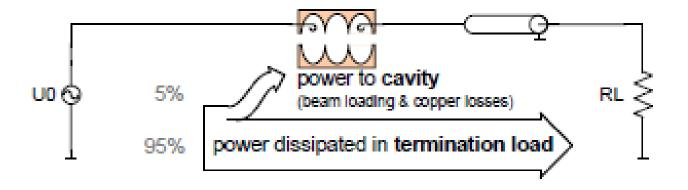
In many particle accelerators considerable amounts of RF power reaching the megawatt level are converted into heat in dummy loads. For the energy recovery, they built two working laboratory prototypes.
