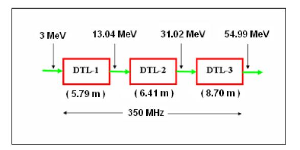
The design of the DTL was started with a 3 MeV input energy and by using three tanks, 55 MeV output energy was achieved.
