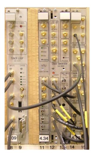
modified LHC hardware: four channels analog down conversion to IF  $f_{RF} = 704.4 \text{ MHz}$  $f_{LO} = (39/40) f_{RF} = 686.79 \text{ MHz}$  $f_{IF} = f_{RF} - f_{LO} = 17.61 \text{ MHz}$
