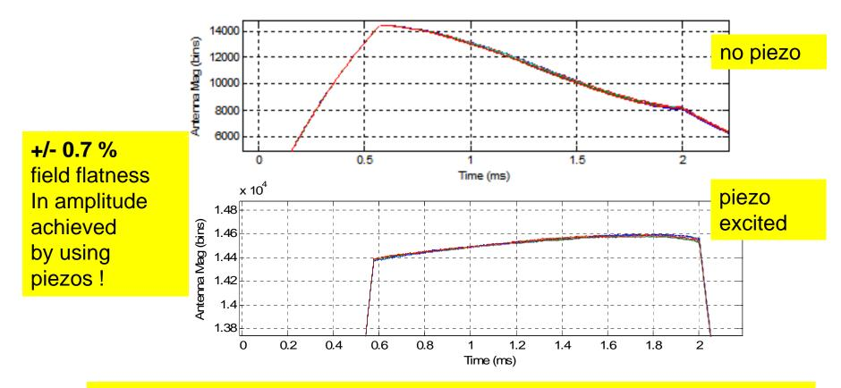
use of piezo minimizes additional RF power needed to further improve the field flatness to the design target of +/- 0.5 %
