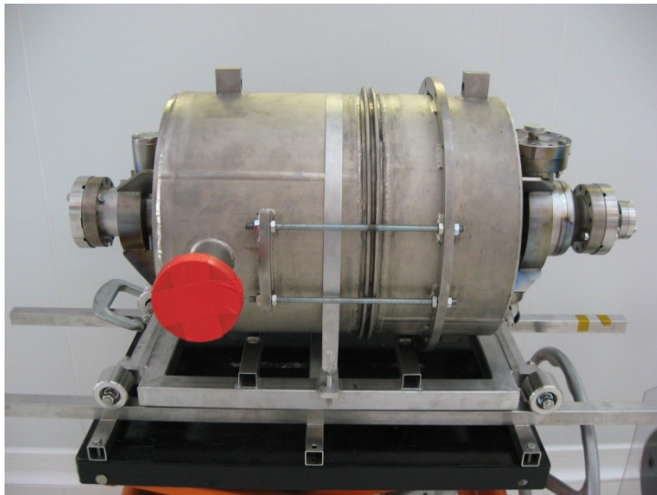
Diameter of the cavity flange (80 mm) NbTi flange with Al hexagonal gasket
