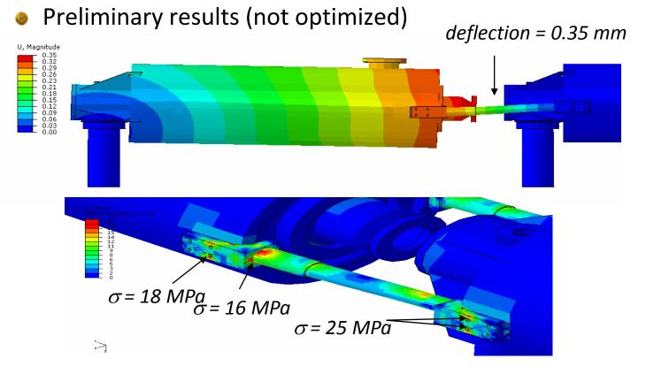
⇒ Small stress (elastic domain) ; but shear stress in the screws
