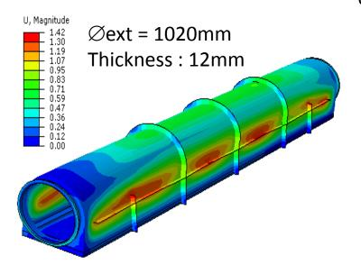
Maximum displacement on the coupler flanges : 0.12mm
