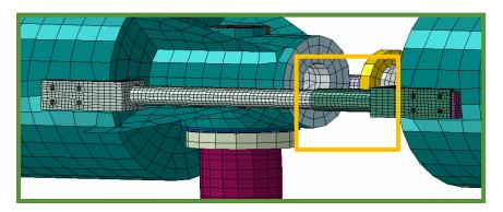
Possibility of adding 2 chocks for the y and z alignment procedure
