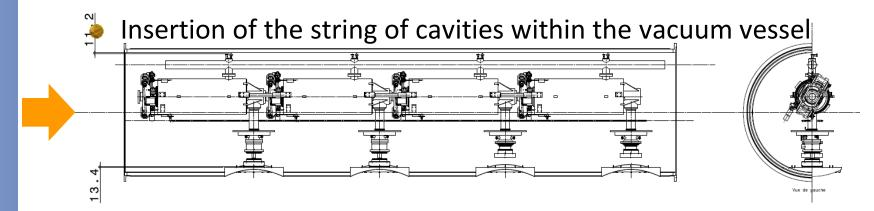
Vertical positioning of the string within the vessel
