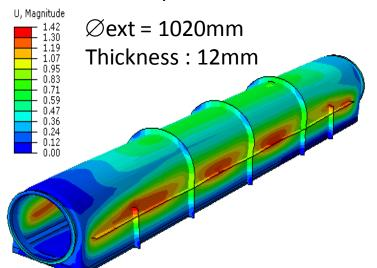
Maximum displacement on the coupler flanges : 0.12mm
