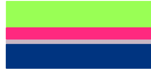
2. wafer + coating, photoresist
