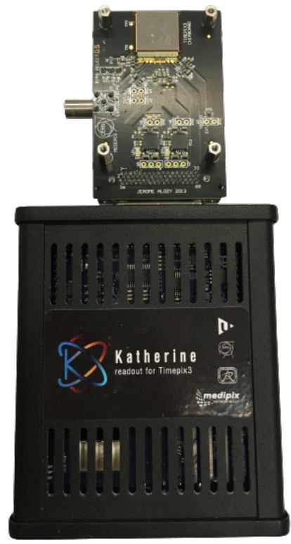
Figure: HR GaAs:Cr-Timepix3 detector with readout interface Katherine.
