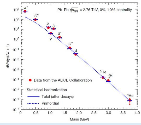
→ In Pb-Pb collisions, particle yields of light flavor hadrons are described over 9 orders of magnitude with a **common** chemical freeze-out temperature of  $T_{\text{chem}} \approx 156 \text{ MeV}$ .
