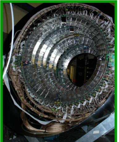
**CHIMERA**: 8 (2x4) rings, high granularity CsI(Tl), 352 detectors  $7^\circ < \Theta < 20^\circ$  + 16x2 pads silicon detectors. Light charged particle identification by PSD. Multiplicity, Z, A, Energy: impact parameter and reaction plane determination
