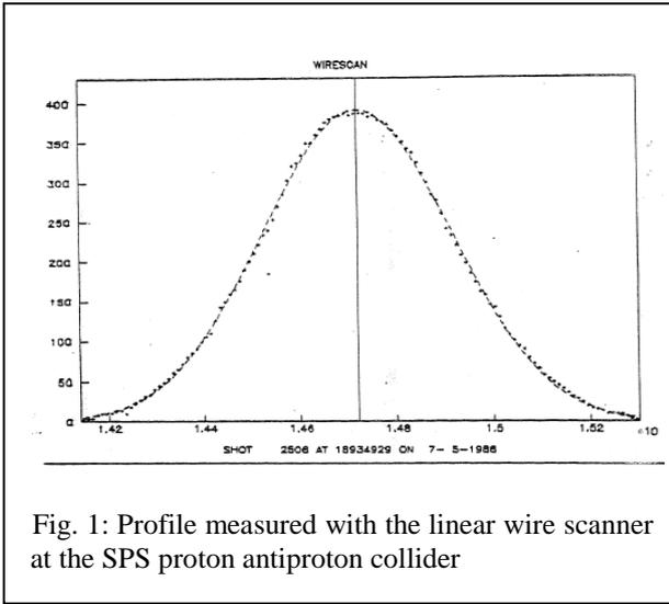
In general, Gaussian beams are assumed. This was shown to be very accurate [8] – the r.m.s. beam size is an excellent assumption for any realistic beam distribution. For precise measurement of the beam profile at the SPS with an error better than 0.5% a linear wire scanner was developed. The result of such a scan is shown in Fig.1. The same type of (linear) wire scanner is also used in LHC. It should also be possible to use these instruments for luminosity calibration at LHC.
