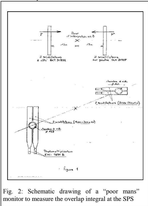
Fig. 2: Schematic drawing of a “poor man’s” monitor to measure the overlap integral at the SPS
