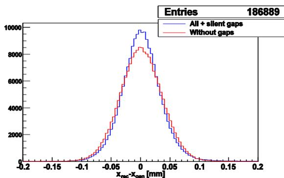
Fig.3 Typical resolution of an ALFA fibre detector.
