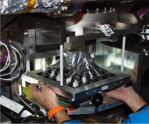
Fig.5: Insertion of a lower fibre detector in the RomanPot.
