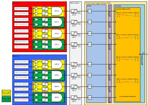
Fig.8: ALFA main trigger logic for elastic scattering.
