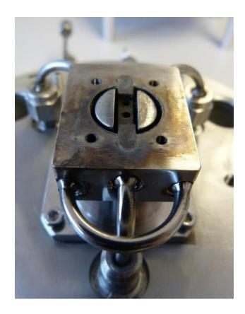
Science and Technology Facilities Council The discharge is sustained by electron emission from the cathodes and ionisation of Cs and H<sub>2</sub> by the "primary electrons".
