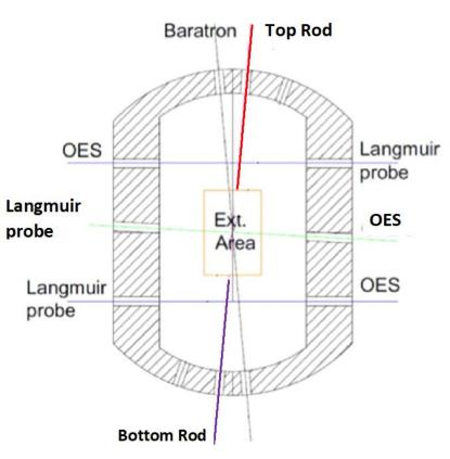
Diameter of the top and bottom rods ~ 8mm and L=250mm Capability to bias the top, bottom and PG independently
