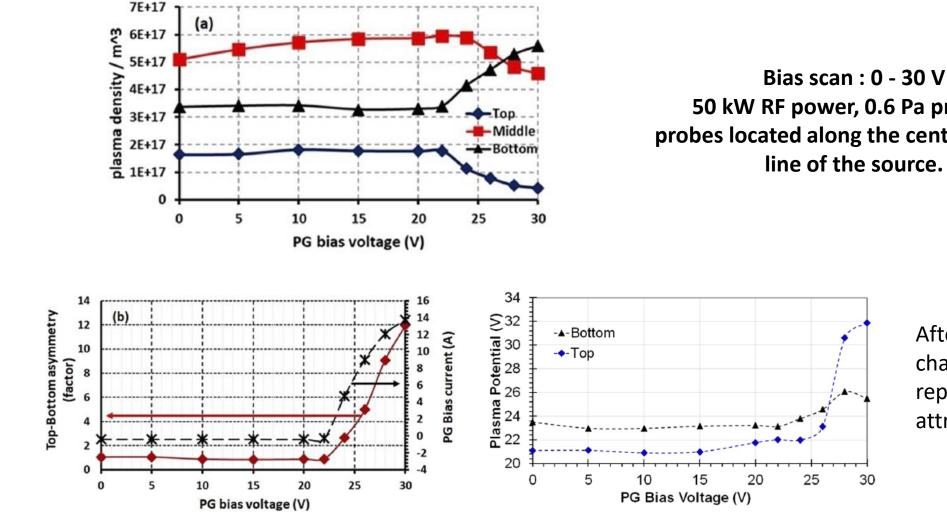
50 kW RF power, 0.6 Pa pressure probes located along the central vertical line of the source.
