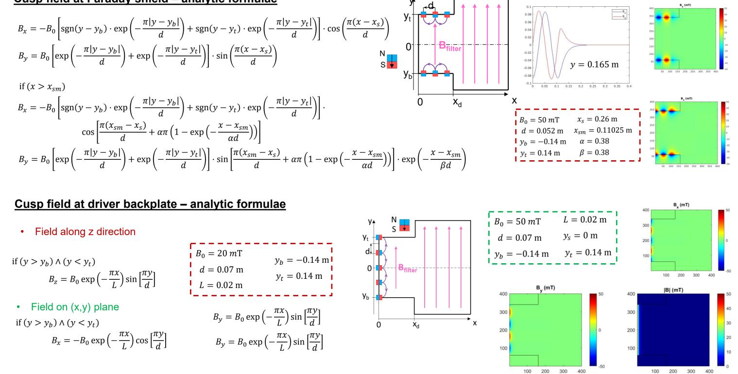
field  $0 \le B_{max} \le 3\text{mT}$  ( $B_{min} = 0.4B_{max}$ ) in order to see the effect of the filter field on the density in the driver. We plot differen x positions , x=8 cm (middle of the driver region) and x = 36 cm (expansion region close to the PG). It can be seen that after initial deacrese, the density increases with the magnetic field in the driver. The density in the expansion region is only marginally affected by the changes to the MF.
