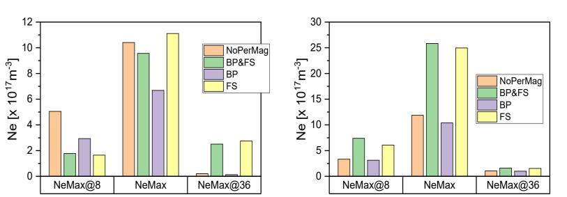
Influence of different permanent magnets configurations on plasma parametrs in SPIDER
