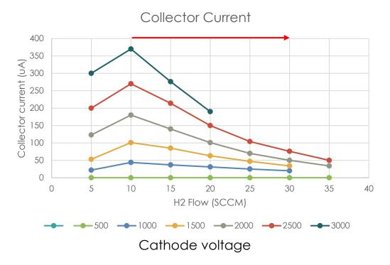
• Probe data shows optimum output at 10 SCCM indicating operation there near the Stoltow point of the Paschen discharge.
