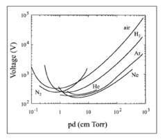
Figure 2.3: Paschen Curve for parallel plate arrangement in various gases (Raizer, 1991. Appeared in Schütze *et al.*, 1998)
