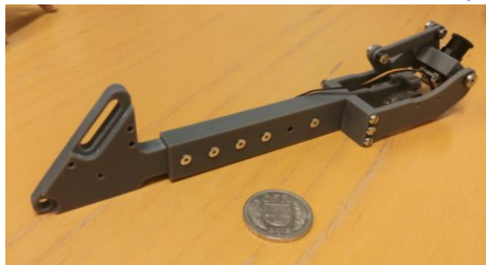
Design, FEM analysis and 3D printing prototype for the RF cavity inspection robot
