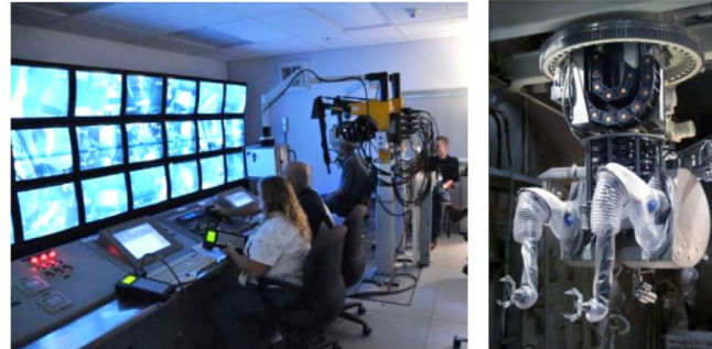
Remote handling control room and the Telerob EMSM 2B tele-manipulator system in use at SNS
