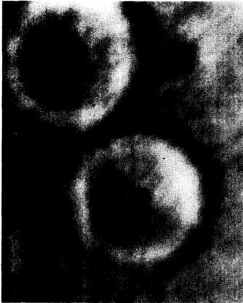
Fig. 11. Laser-produced arc crater. Rim-to-rim diameter is 5.5 \mu\text{m} , and the cathode spot size is 0.7 \mu\text{m} .
