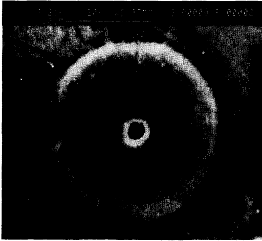
Fig. 10. Unipolar arc crater on the cathode surface.
