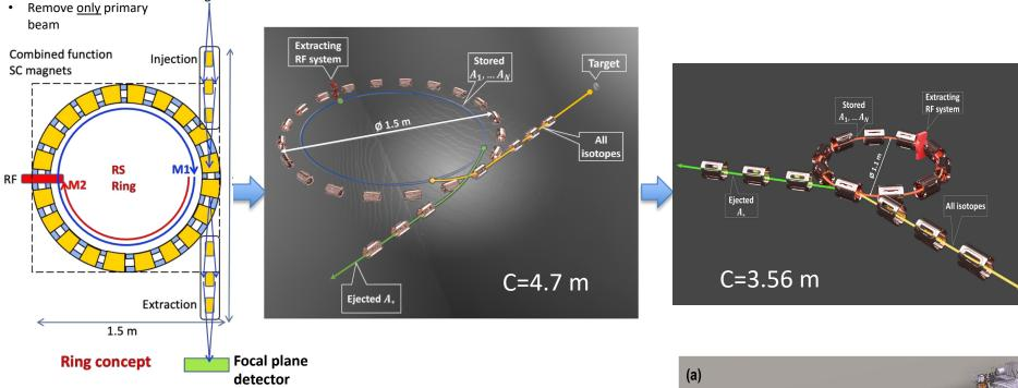
Based on combined function magnets: dipolar and qua Maximum magnetic field ~ 6 T
