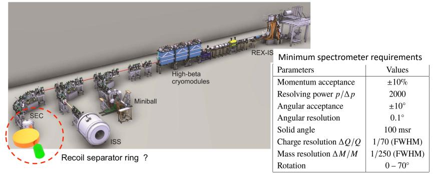
A compact recoil separator can bring new and exciting possibilities to the HIE-ISOLDE physics program
