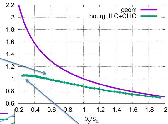
For flat beams, the optimum is around  $\beta_v$  $= 0.25 \times \sigma_{7}$
