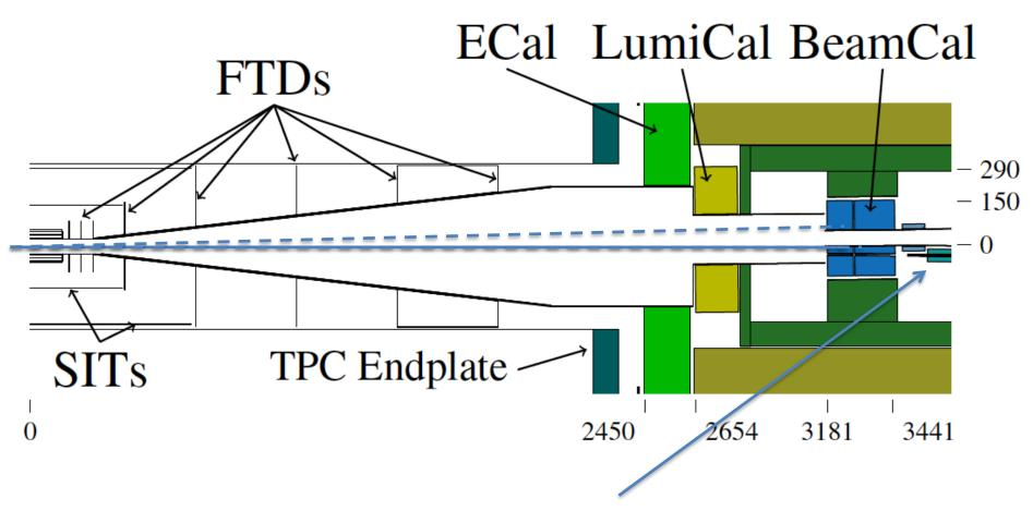
The last focusing magnet of the machine is inside of the detector
