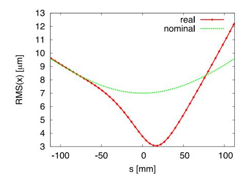
Electron beam shrinks during collision Increases beam-beam tune shift for protons
