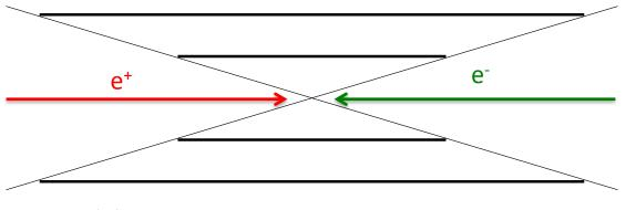
Hit density from pairs depends on radius and field Edge is due to beam-beam deflection
