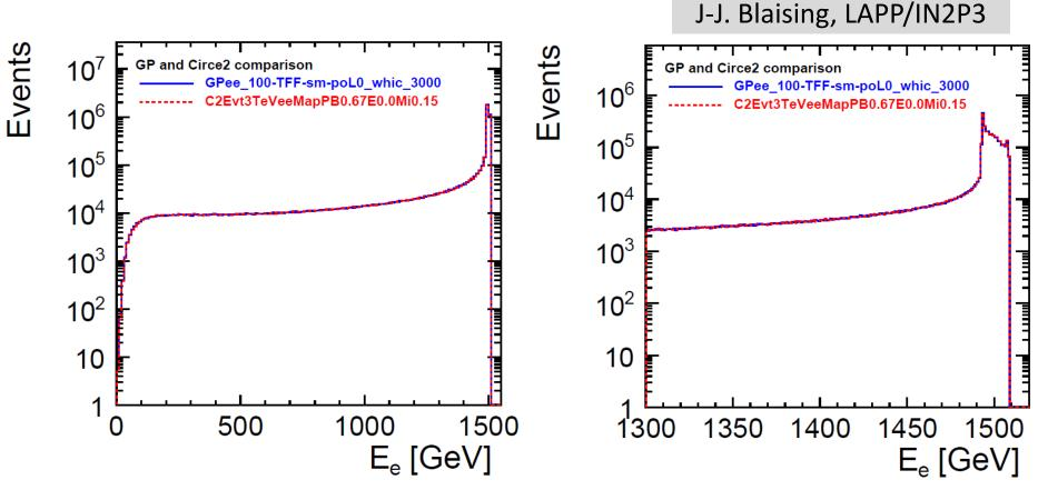
Left: dN/dEe distribution Guineapig events (blue) and Circe2 generated events using a Power function mapping (red); 20 GeV bins.
