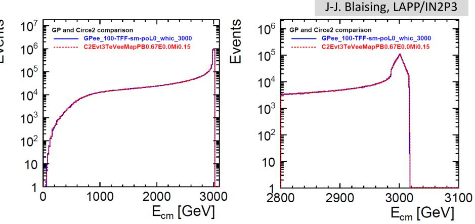
Left: dN/dVs distribution Guineapig events (blue) and Circe2 generated events using a power function mapping (red); 20 GeV bins.
