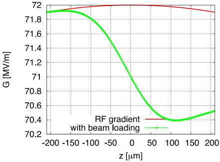
Loaded gradient seen by a single bunch for off-crest acceleration (12°):
