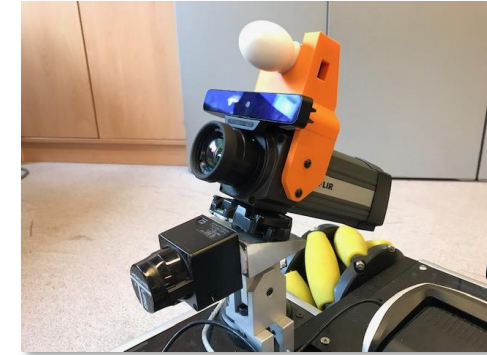
Vision system (2D Laser, radar, thermal and 2D-3D camera)
