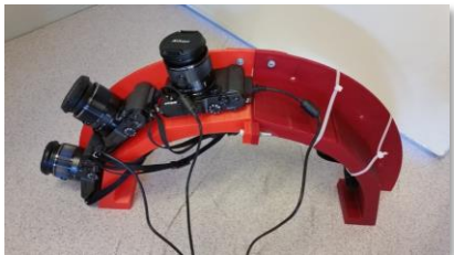
HD camera system for tunnel dome view
