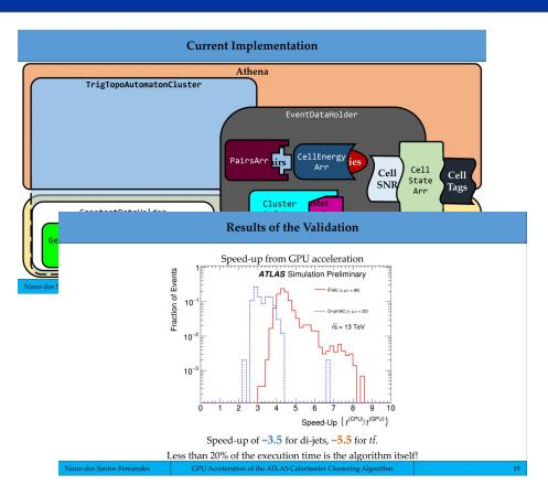
One successful recent demonstrator was written for reconstructing clusters of energy deposits in the ATLAS calorimeters
