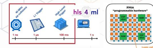
CERN needs ultra fast deep learning inference (execution in ~1 microsec) for fast classification of particle collision data, requiring compact code for edge-computing on programmable chips (FPGAs with logic cells)
