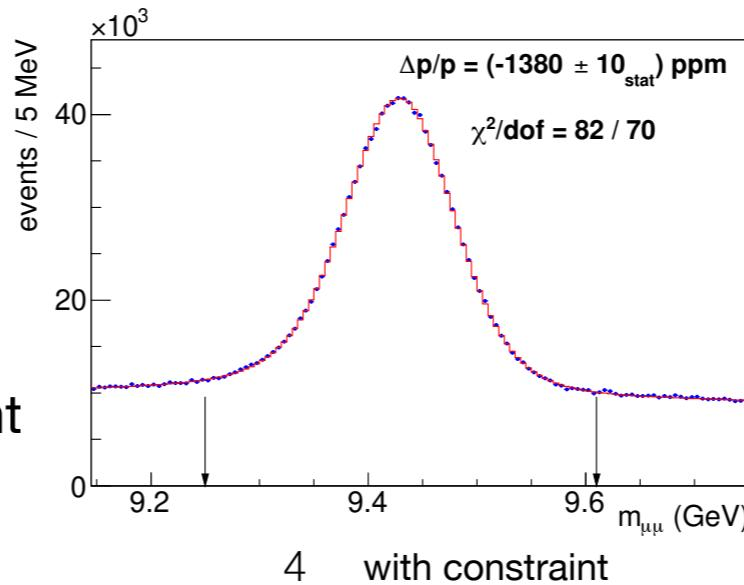
**Third step is the scale calibration from  $\Upsilon$  decays to muons**
