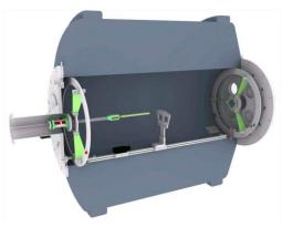
Fewer electronic channels, cheaper, easier to operate. Better solid-angle coverage for the same cost. NB: acceptance largely determined by length of silicon, bore and field of magnet.
