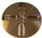
Accelerating structure prototype for CLIC: 12 GHz ( L \sim 25 cm)
