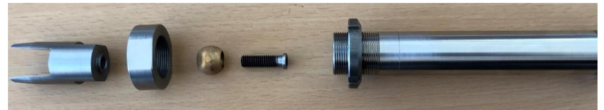
Top: A steel flexure from the adjustment platform and the fully assembled test joint. Bottom: The test joint disassembled, showing a spherical bearing.
