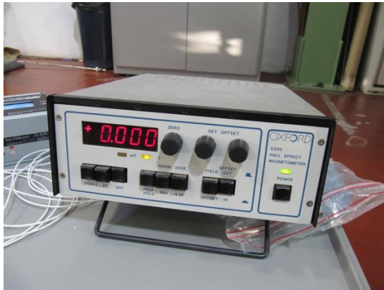
Magnetic measurements were done manually after each PM was inserted. Results were very close to simulations.
