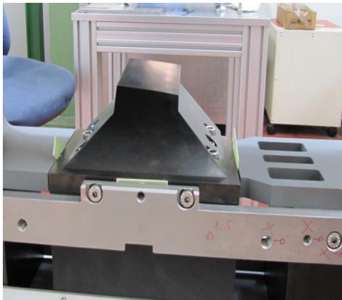
All the poles were fixed in their nominal position using gauges
