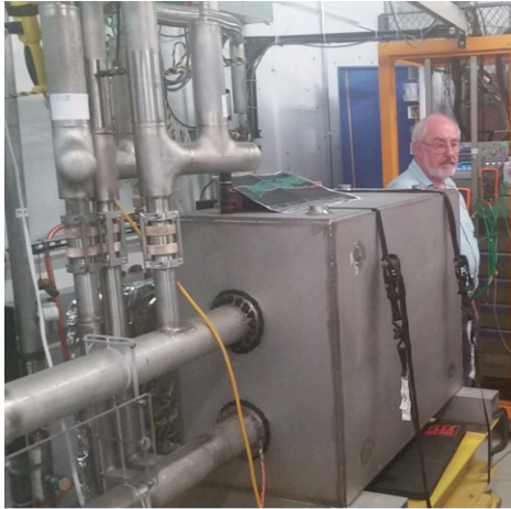
Test of fast-ramping normal-conducting magnet design
