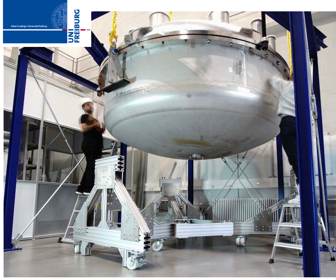
Test electrodes with 2.6 m diameter
