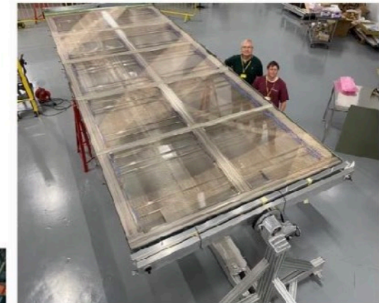
APAs for Module 0 ProtoDUNE being tested at Daresbury Laboratory, UK. One 2.3m x 6.3m APA is shown; UK to provide 130 APAs.
