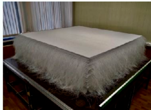
2 million scintillator cubes assembled
