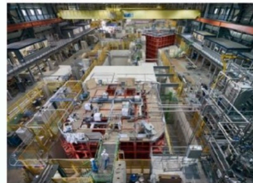
NP-02 and NP-04 ProtoDUNE 8m x 8m x 8m detector prototypes at CERN.
