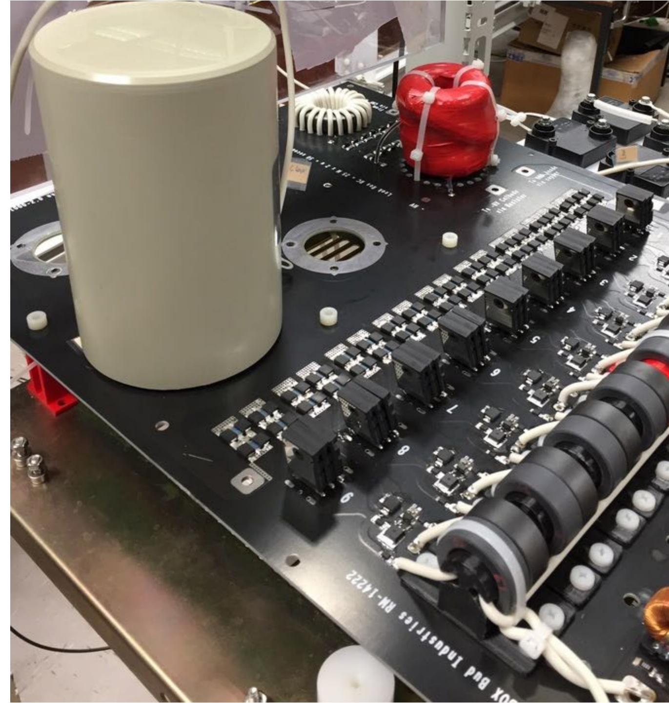
>> high-power compact robust flyback transformer for up to 120 kV
