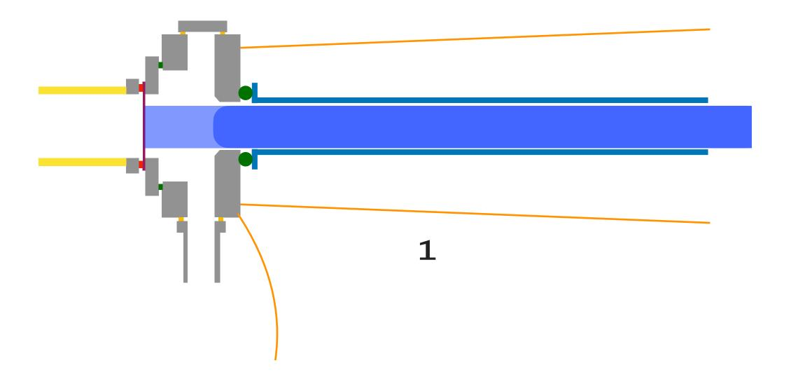
> conductance is required between tube and vacuum/gas system > foil is required to separate 1-10 Pa argon/xenon in tube and vacuum in pipe > glass tube should end when it meets the metal > plasma should have well defined density (avoid ambiguous extremities) > vacuum separation foil is 100 um Al
