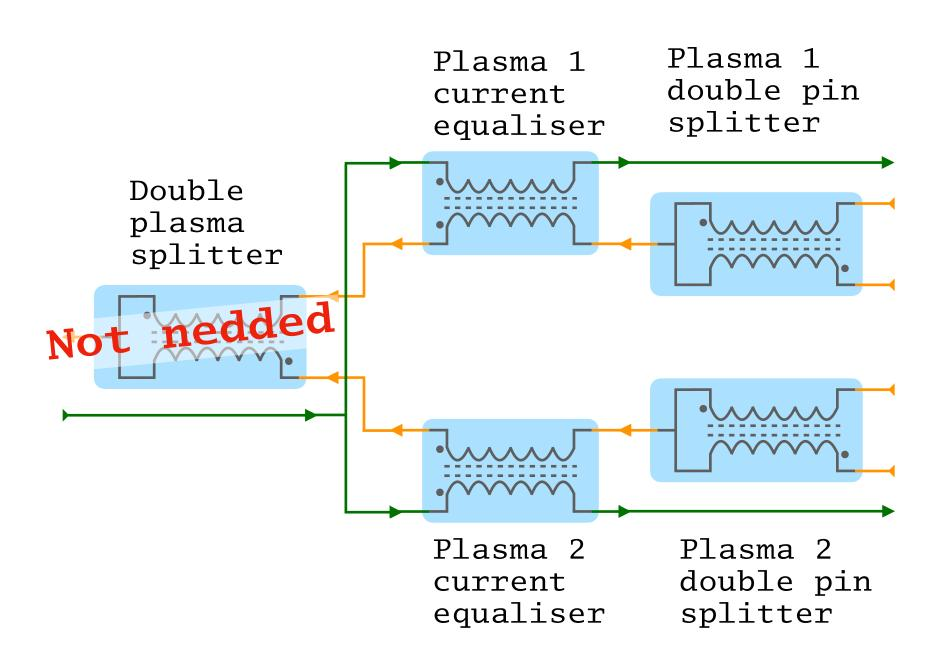
>> CBM for a double plasma with a common 4 pin cathode
