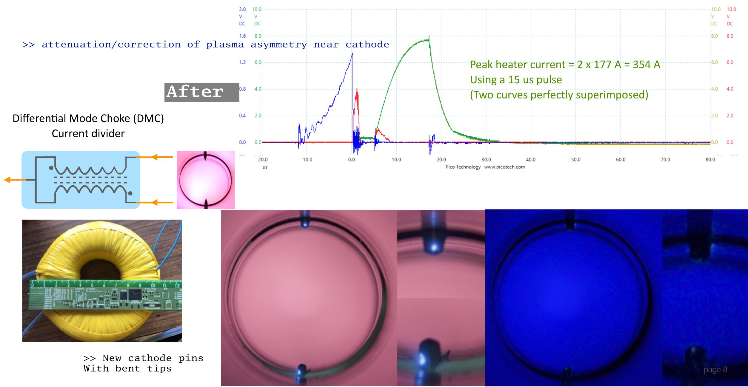
>> Full fast risetime CBM for 4 pin common cathode and **double plasma** in asymmetric tube (2m + 3m)
