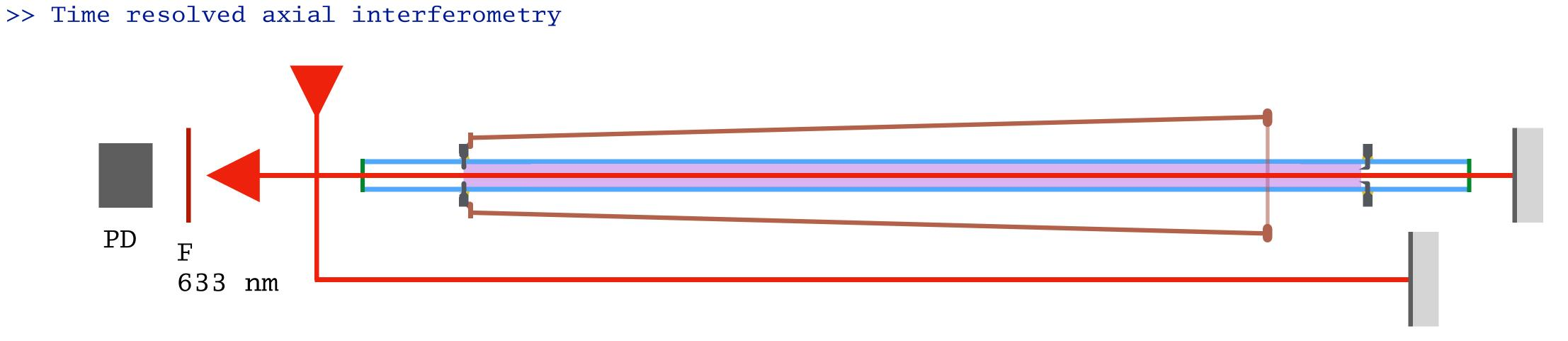
Essential diagnostic to balance > 1 plasma Used at IST with He:Ne laser with ~ 5 % precision so far Plan to improve SRN and reach ~ 2 % Plan to implement quadrature measurement to reach < 1 %
