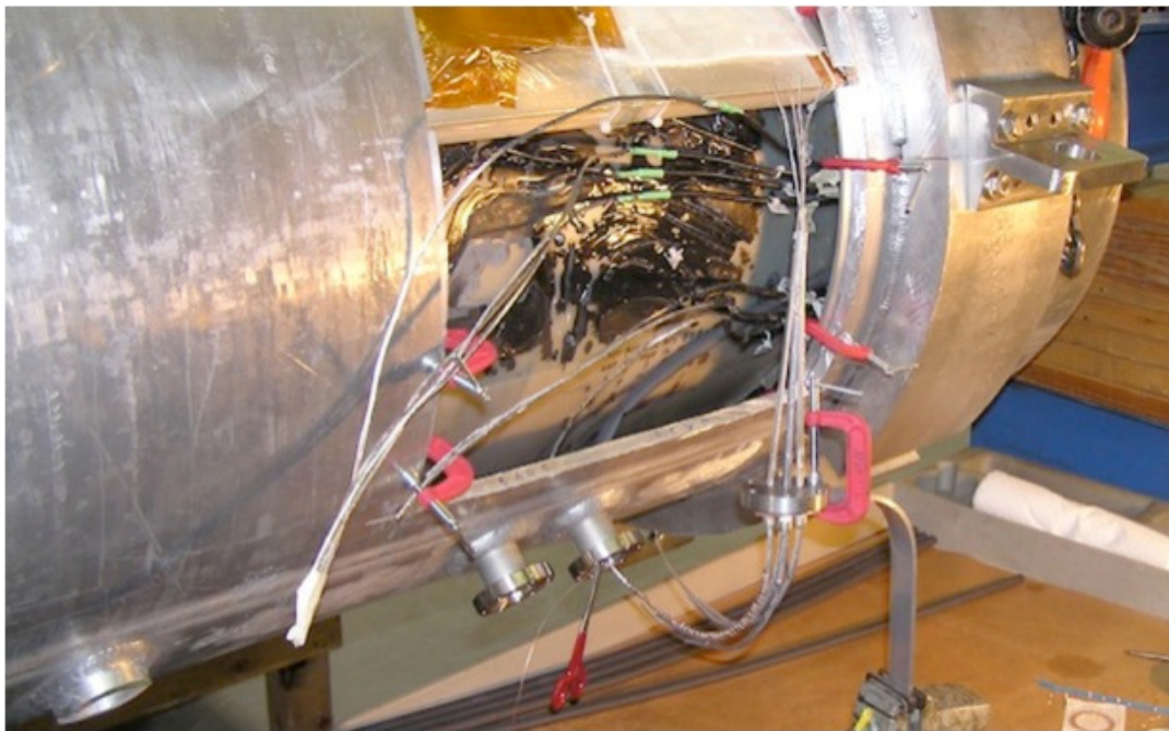
Figure 6: Repair and stabilization of the Magnet 2B cold leads.
