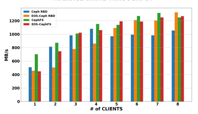
EOS+Ceph has a better throughput than Ceph, as the number of clients increases
