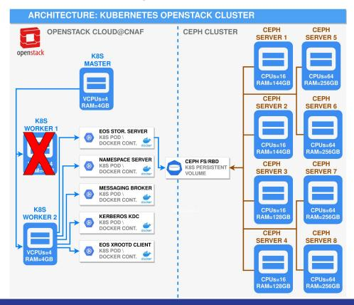
If a K8S worker node is shut down, simulating a failure, and then removed from the cluster, EOS Pods automatically migrate
