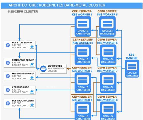
Ceph cluster nodes used to host a K8S cluster
