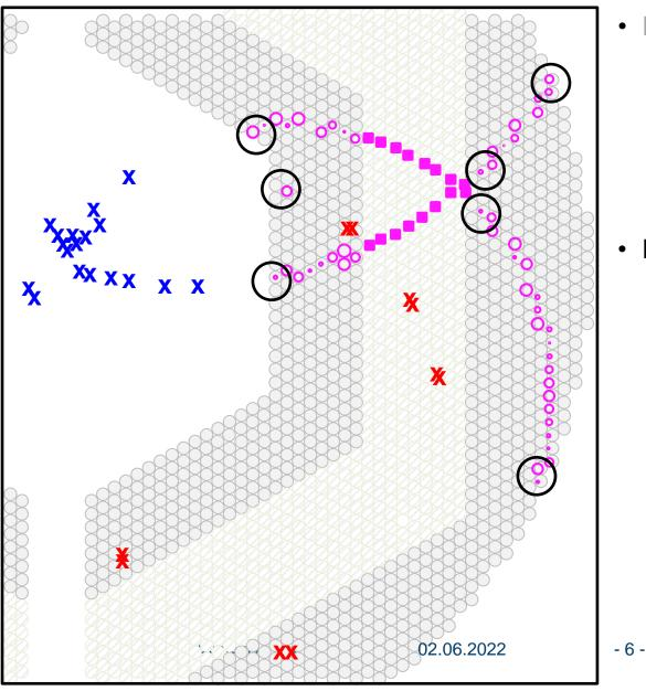
→ Tracks originating from displaced secondary vertex
