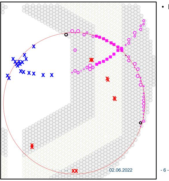
→ Tracks originating from displaced secondary vertex
