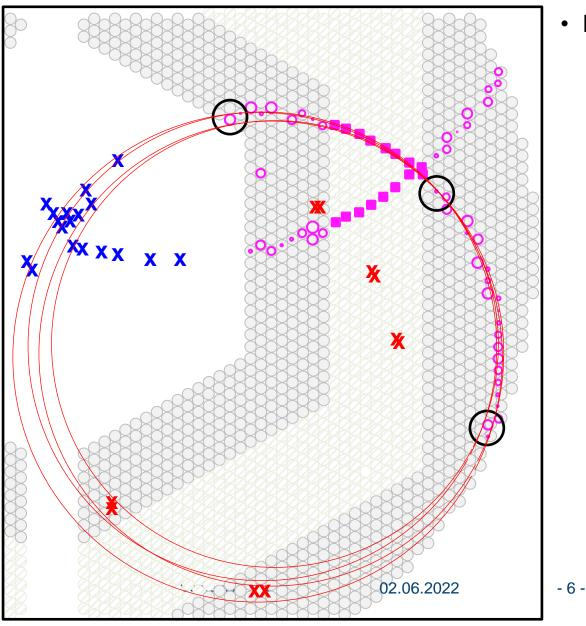
→ Tracks originating from displaced secondary vertex
